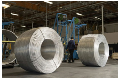
Figure 10: Spools of next generation TS Conductor
